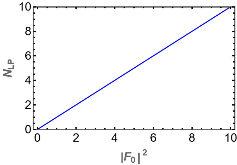
Varying the pump amplitude for fixed pump frequency ( $\omega_p = \omega_{LP}$ ).
